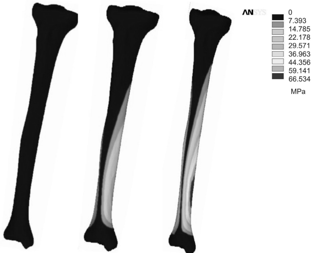
Fig. 4. Stress distribution in health tibia for the applied loading: a) 100 N, b) 1000 N, c) 2000 N
