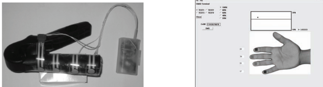
Figure 3. The CustoMed architecture applied to a neurological applications (a) hand grip to quantitatively determine the range of motion of patients (b) interface to give doctors and patients feedback during rehabilitation.
