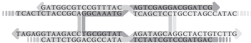
FIGURE 5.15 A schematic DNA structure for creating “tiles” that can join other tiles. (Adapted from Barish, Robert D., Paul W. K. Rothemund, and Erik Winfree, Nano Lett 5, no. 12, 2586–2592, 2005. With permission.)
