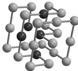
Fig. 1. One of the 103346 possible compact conformations of sequence \text{PHP}_4\text{HPHPHP}_{15}\text{H} . The hydrophobic (H) residues are the darkest ones.
