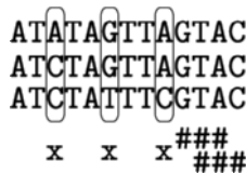
Figure 15.2 Words belonging to a (13, 3, 2) -Hrepeat share at least p_3 nonoverlapping 3-grams with p_3 = \left\lfloor \frac{13}{3} \right\rfloor - 2 - (3 - 2) \times \left\lfloor \frac{2}{2} \right\rfloor = 1 . Indeed, a 3-gram GTA, for instance, is shared by the three sequences. In this example, mismatches were spread every three characters. This repartition is the most limiting case for the number of shared 3-grams.
