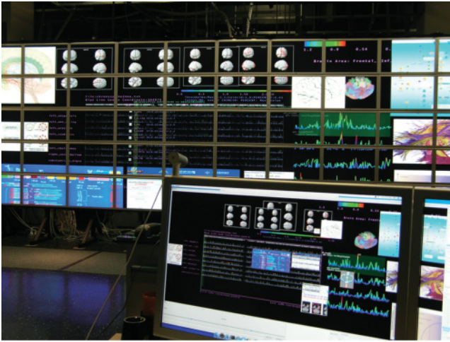
Figure 27.5 Scalable imaging genetics workspace allowing data to be processed through user-centric view and shared visual analytics space, the wall.
