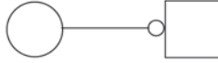
Figure 2. Three equivalent graphical representation for read or test arcs. Read arcs form loops. They can be used to model catalysts, because catalysts, e.g., enzymes, are necessary for the occurrence of a biochemical reaction, but will not be consumed during the reaction.
