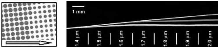
Fig. 17. Flow device in which the asymmetric disposition of obstacles is achieved by tilting the axes of a regular lattice at a slight angle to the flow. By grading the size of the gaps between the obstacles over the range 1.4\ \mu\text{m} - 2.0\ \mu\text{m} , particles of sizes 0.8\ \mu\text{m} , 0.9\ \mu\text{m} and 1.0\ \mu\text{m} can be made to depart from the main flow direction at different locations.
