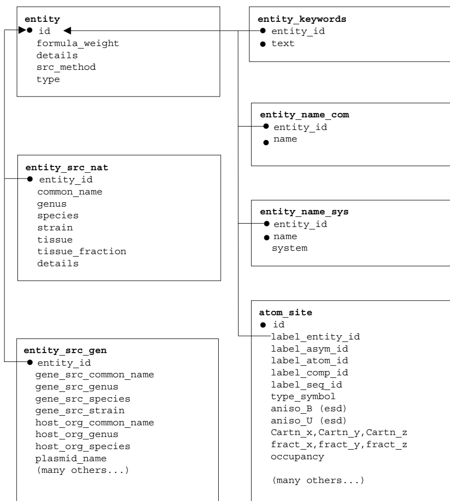
Figure 8.9. A schematic diagram illustrating the content and relationships among a portion of the mmCIF categories describing chemical entities, entity names, entity source organism, and the relationship between the entity and atomic level of description. In this figure, boxes enclose the data items within each mmCIF category, and arrows indicate the correspondence between data items that are common to multiple categories, with the arrowheads pointing in the direction of the parent data item. The category key data items are indicated with black dots.
