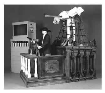
**Figure 19** In this virtual reality system, a platform with a ship's wheel mounted on it provides the space where the participant takes their virtual voyage. (Image courtesy Randy Sprout.)
