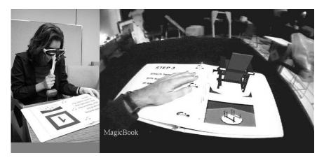
**Figure 5** A children's book or an instruction manual can come alive through the "magic book" augmented reality concept. Here, the steps of how to assemble a chair are explained and demonstrated by looking through a head-based display system that augments the contents of the book. (Image courtesy University of Washington at Seattle.)
