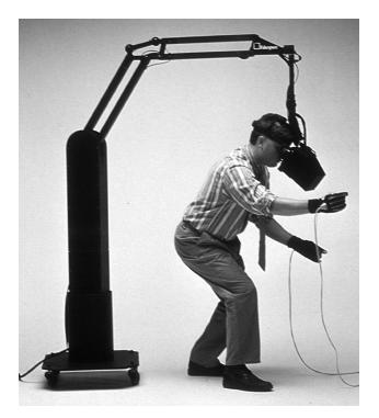
**Figure 12** The BOOM head-based display mounts the screens on an arm that takes the weight from being applied to the user's head. (Image courtesy Fakespace Systems, Inc.)
