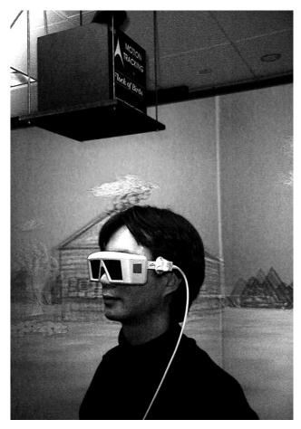
**Figure 17** A low-level electromagnetic field is emitted by the large black box. The signal is sensed by a recieving antenae which allows the system to determine the location and orientation of the receiver. (Copyright 2003, William Sherman.)
