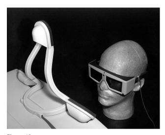
**Figure 18** This basic ultrasonic tracking system uses three speakers and three microphones triangularly arranged to measure the distance between all the speaker–microphone pairs from which the location and orientation of the glasses can be determined. (Copyright 2003, William Sherman.)
