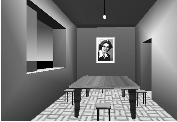
Figure 7 Perspective view of a CAD of a room, rendered with shading, textures, and transparency.
