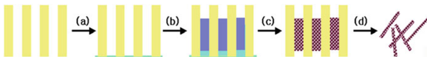
Fig. 4.11 Schematic diagram of the fabrication of nanoporous Au nanowires. (a) Ag sputtering; (b) electrodeposition of Ag and Au–Ag alloy nanowires into the alumina membrane; (c) chemical dissolution of Ag electrodes and Ag from the Au–Ag alloy nanowires by concentrated nitric acid; and (d) alumina removing in NaOH solution
