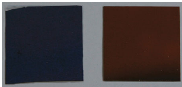
Fig. 13.24 Photographs of nanodome solar cells ( left ) and flat film solar cells ( right )
