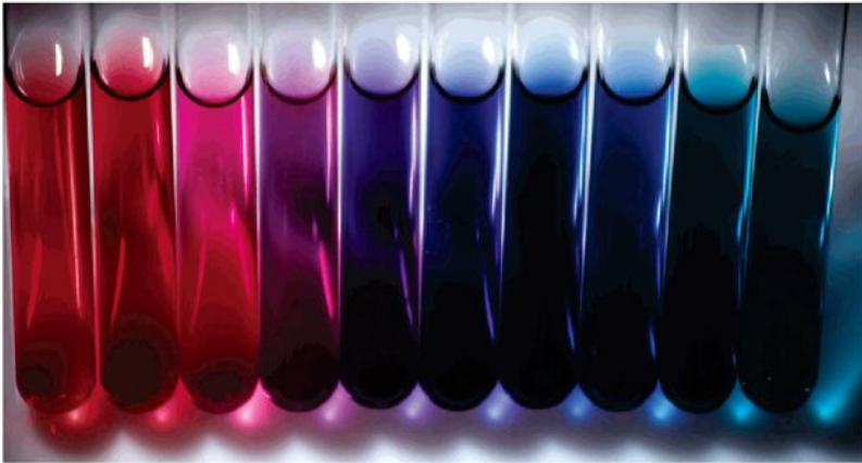
Fig. 1.2. (a) UV-visible absorption spectra of nine hollow gold nanosphere (HGN or HAuNS) samples with varying diameters and wall thicknesses. (b) Photograph showing the different colors of HGN solutions in different vials. The vial on the far left contains solid gold nanoparticles, the rest are HNGs with varying diameters and wall thicknesses. Reproduced with permission from Ref. 2.
