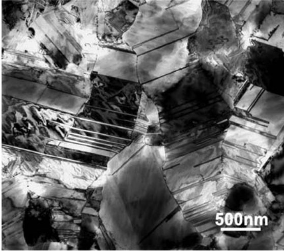
Fig. 19.15 Transmission electron micrograph of a nanotwinned Cu, showing a high density of growth twins inside sub-micrometer-sized grains. The material was prepared through electrodeposition. By adjusting the deposition parameters, different twin densities can be achieved.
