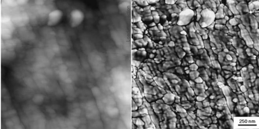
Fig. 4.11 An AFM topograph (left) taken from the surface of an HPT-processed Ti sample after being tested in tension at 250°C for a strain about 30% (see curve 3 in Fig. 4.10). The right micrograph is a derivative of the left one [102].
