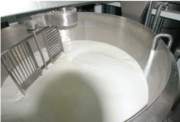
FIGURE 1.2 Yogurt culture addition in a tank.
