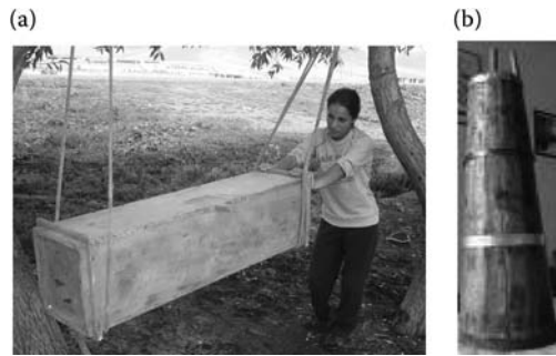
FIGURE 4.4 Wooden barrel churns: (a) horizontal type and (b) vertical type.
