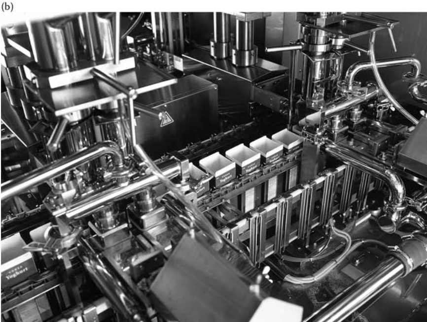
FIGURE 2.11 (a) External and (b) internal appearance of Pure-Pak P-S50S-med filling machine. (Reproduced with permission from Elopak AS, Skjerve.)
