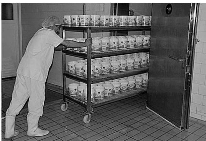
FIGURE 1.8 (See color insert following page 212.) Yogurt containers on the shelves of an incubation room at 42–43°C.
