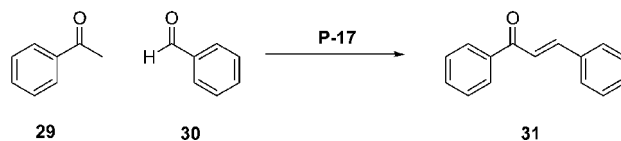
Scheme 13 Schematic representation of molecularly imprinted polymer preparation for P-17 and subsequent use to catalyze the aldol condensation between acetophenone, 29 , and benzaldehyde, 30 .
