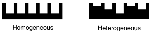
Figure 1 Schematic depictions of homogeneous and heterogeneous MIPs that contain binding sites in which the sites are identical or different. The depth of the site corresponds to the binding affinity.
