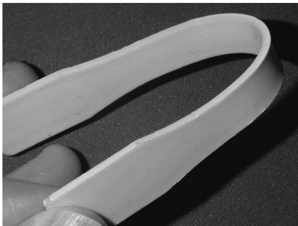
Figure 5.5 Demonstration of the flexibility of 70% \text{CaCO}_3 ( 2.5 \mu\text{m} ), 0.5% KR TTS-treated filled PP homopolymer. Untreated 70% \text{CaCO}_3 -filled PP would snap and break at the slightest deformation.
