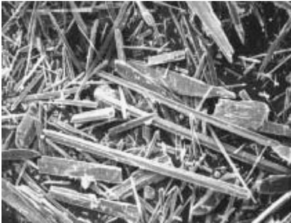
Figure 14.1 Microphotograph of acicular wollastonite (VANSIL ® WG, R.T. Vanderbilt Co., Inc.), 170 \times .
