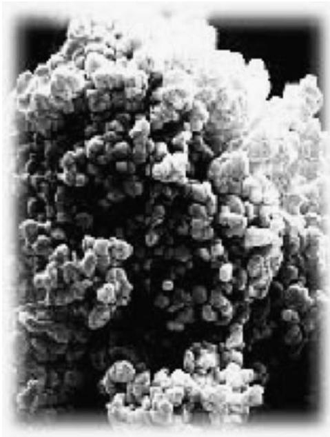
Figure 20.1 A typical SEM of “light-burned” MgO submicron particles with surface area 0.1–1.0 m 2 /g. Reproduced with permission from Ref. [3].
