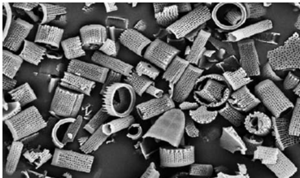
Figure 19.7 An example of a DE deposit with a single principal Diatom present, 1000 \times . Courtesy of World Minerals Inc.
