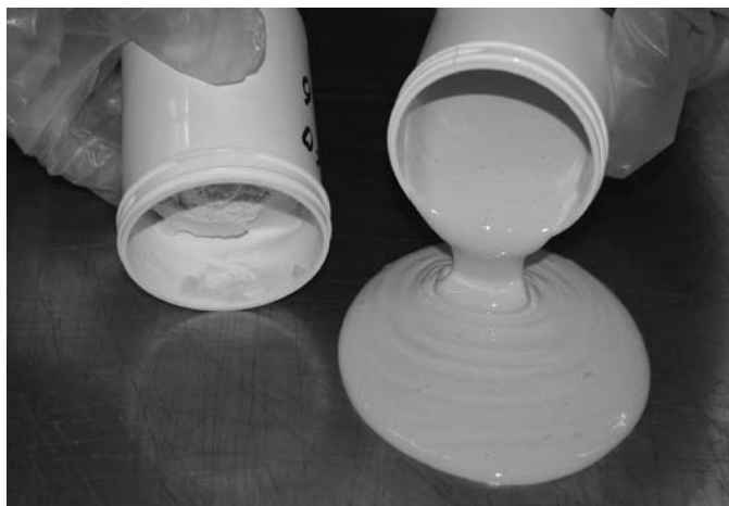
Figure 5.8 (Left) 40 wt% calcined clay in mineral oil – 2 000 000 cps viscosity. (Right) 0.7 wt% LICA 38 of calcined clay added in situ to mineral oil followed by 40 wt% clay – 9200 cps viscosity.
