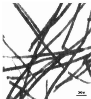
Fig. 6. SEM image of Ni nanorods nanowires from a colloidal suspension.
