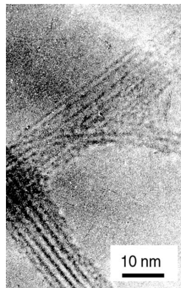
FIGURE 2. HRTEM image of arc-produced SWNT rope .
