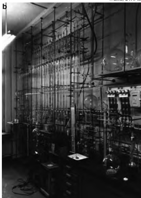
Fig. 8.9 (a) A four stage thermal diffusion cascade for argon isotope separation (Modified from Spindel, W. ACS Symp. Ser. 11 , 82 (1975)). (b) The thermal diffusion cascade operated by K. Clusius and collaborators at the University of Zurich during the 1950s (Photo credit: Archives of the Institute of Physical Chemistry, University of Zurich)
