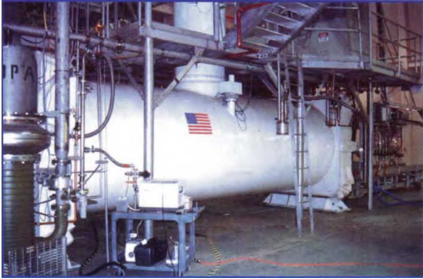
Fig. 8.7 The PSP Superconducting Ion Cyclotron Resonance Isotope Separator. The large tank holding the superconducting magnetic is \sim 15 m long \times 2 m diameter (Reprinted from Bigelow, T. S. et. al. Nucl. Instr. Methods Phys. Res. B 241 , 652 (2005), copyright 2005 with permission from Elsevier)
