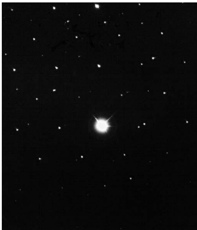
FIGURE 11.1. An experimentally observed DP showing the central, intense, direct beam and an array of diffraction spots from different atomic planes. Such a pattern, with sharply focused spots, is best obtained by underfocusing the beam.
