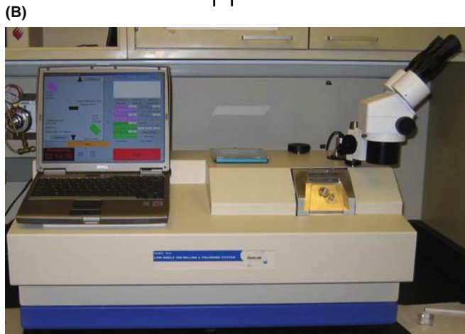
FIGURE 10.9. (A) Schematic diagram of an ion-beam thinning device: Ar gas bleeds into an ionization chamber where a potential up to 6 keV creates a beam of Ar ions that impinge on a rotating specimen. Although not shown, the whole apparatus is under vacuum. The specimen may be cooled to liquid-N 2 temperatures and perforation is detected by the penetration of ions through the specimen. (B) Typical ion mill.
