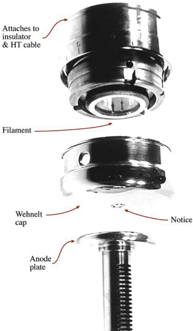
FIGURE 5.2. The three major parts of a thermionic gun, from top to bottom: the cathode, the Wehnelt cylinder and the anode shown separated. The Wehnelt screws into the cathode support and both are attached to the high-voltage cable which also contains power supplies for heating the cathode and biasing the Wehnelt. The anode sits just below the Wehnelt and the whole assembly sits on the top of the column of lenses that make up the rest of the TEM.
