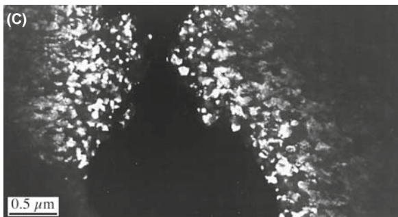
FIGURE 18.10. (A) A textured ring pattern where the rings are more intense over a certain angular range. (B) The corresponding interception of the Ewald sphere (plane) with the reciprocal lattice. (C) A DF image of the textured grains, taken from a brighter portion of one of the hkl rings, showing an equiaxed structure. In (D) the specimen is textured about a direction at an angle to the beam, so the Ewald sphere creates elongated spots or arcs in the DP (E).
