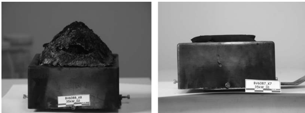
FIGURE 15.12 Fire residue of EP+15 wt.% APP (left) and EP+LS+10 wt.% APP (right). Combining APP with LS inhibited intumescence, causing strong antagonism.
