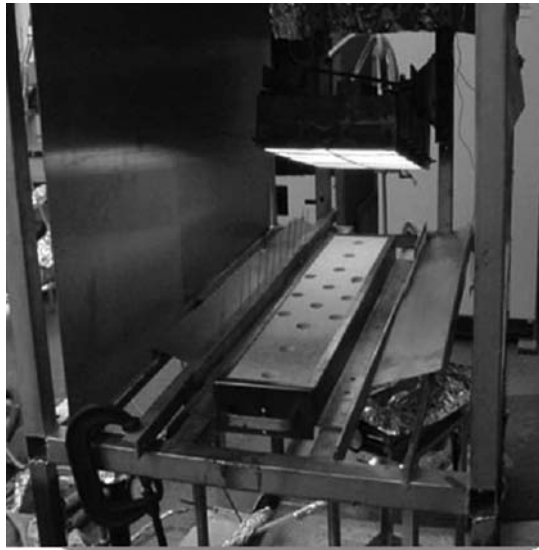
FIGURE 16.11 RPA with a gas radiant heat source and a ceramic sample holder.
