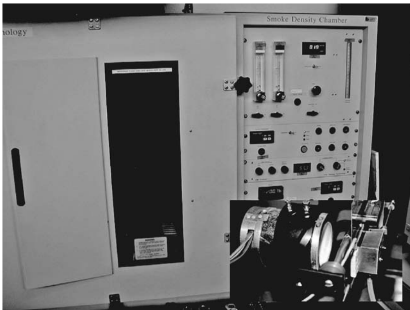
FIGURE 14.12 NBS Smoke density chamber with heater described in IMO FTP code. Insert: Close-up view of ASTM E 622 heater. (Photo courtesy of Southwest Research Institute, San Antonio, TX.)
