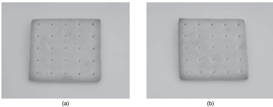
Fig. 4.4 (a) Semisweet biscuit prepared in lab bakery: control, no asparaginase addition. (b) Semisweet biscuit prepared in lab bakery: asparaginase treated.
