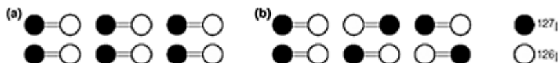
Fig. 3. (a) The only possible ordered arrangement of six ^{127}\text{I}^{126}\text{I} molecules in a lattice; (b) one of 15 possible arrangements where two of the molecules are reversed.
