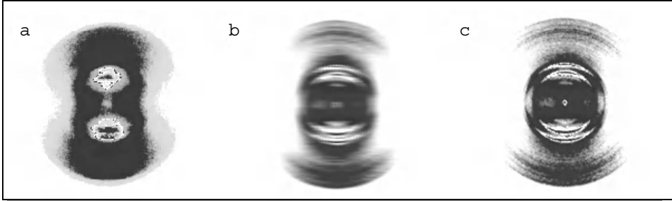
Fig. 2.20. Comparison of ion imaging and velocity mapping images taken under the same conditions. Panel (a) is ion imaging, panel (c) velocity map imaging, and panel (b) shows the effect of cancelling the velocity mapping by smearing the image out along the x direction by 2 mm. This illustrates the extra effect of the grids on lowering the image quality.
