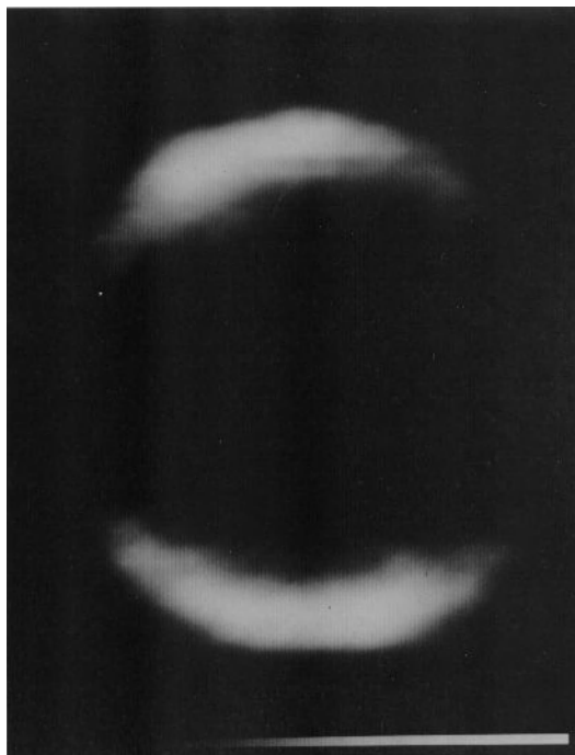
Fig. 1.5. Image of \text{CH}_3(v = 0) fragments produced from the photolysis of \text{CH}_3\text{I} with 266-nm light. The polarization axis of the dissociation light is vertical and in the plane of the figure. Reprinted with permission from Ref. [19]. Copyright 1987, American Institute of Physics.
