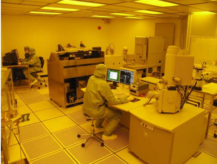
Fig. 4. Photo of the class 1000 cleanroom of SSSL showing the e-beam writer, laser writer, plasma cleaner and hot embosser. The X-ray scanner is in the background, hidden by the laser writer.
