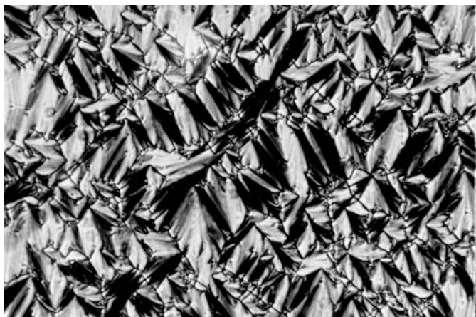
Figure 4.21. Focal-conic fan texture of a smectic A phase.
