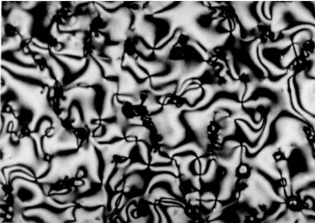
Figure 4.13. Photomicrograph of the schlieren texture of a polymeric nematic phase.
