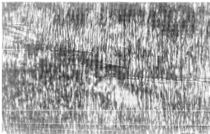
Figure 4.19. Banded texture of a mesogen-jacketed liquid crystalline polymer. The shearing direction is perpendicular to the direction of the parallel bands.
