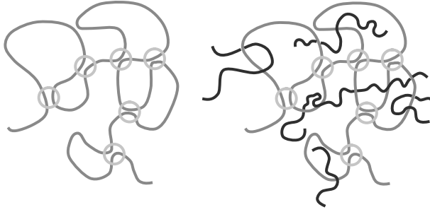
Fig. 3.1. The single chain versus a labeled chain in a melt. The single chain experiences contacts only with itself, whereas the melt chain has contacts with all neighboring chains. Thus the self-contacts, depicted by the circles, become irrelevant as the concentration increases. From [188], reprinted with permission of Elsevier.
