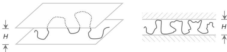
Fig. 6.3. A linear polymer chain between two parallel plates. The polymer chain can be immediately replaced by a chain of any connectivity. For simplicity, only the case D = 1 is shown. Reprinted from [65] with permission from Elsevier.
