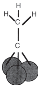
Figure 7.3 Schematic representation of the ethylidyne species formed via reaction of ethene over Pt surfaces
