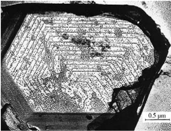
Figure 5.3. Spiral steps observed on the mineral kaolin using transmission electron microscopy with the decoration method [7].
