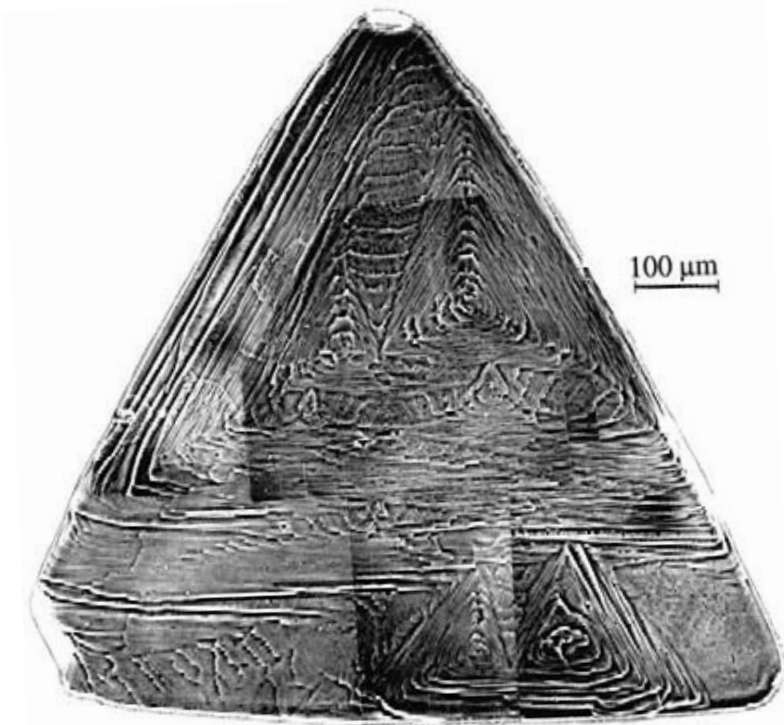
Figure 9.10. Phase contrast photomicrograph of a (111) face of an octahedral diamond crystal from Siberia. Note the triangular pyramidal growth hillocks and small trigons at the summits of the respective growth hillocks. Photographed by K. Tsukamoto [12].
