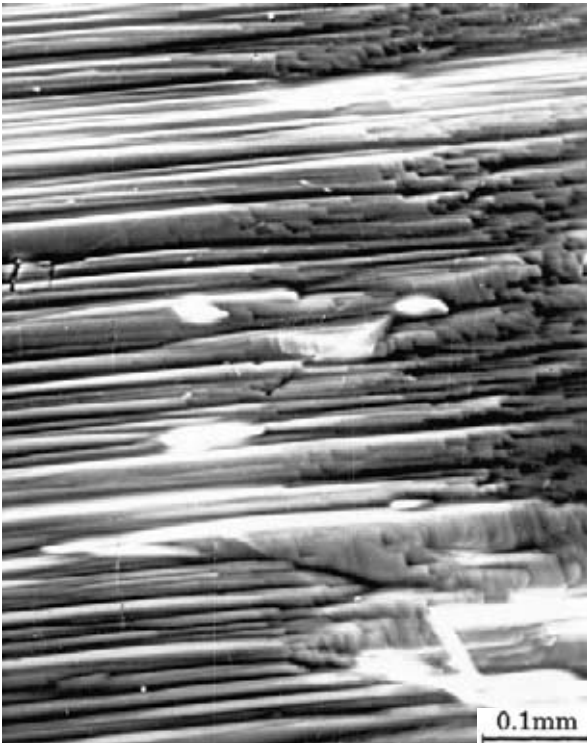
Figure 10.5. (a) Polygonal spiral growth hillocks universally observed on \{10\bar{1}0\} faces of synthetic quartz. (The arrows indicate the summits of the growth hillocks.) (b) Striation patterns commonly seen on the \{10\bar{1}0\} faces of natural and synthetic quartz grown in NaCl aqueous solution.
