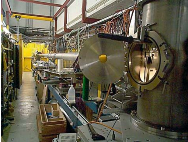
Figure 4.10. Beamline BW4 at HASYLAB. View from a sample chamber along the vacuum tube towards the detector at the opposite yellow wall
