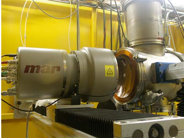
Figure 4.13. mar ® 185 CCD–detector in operation at beamline BW4, HASYLAB at the rear end of the vacuum tube
