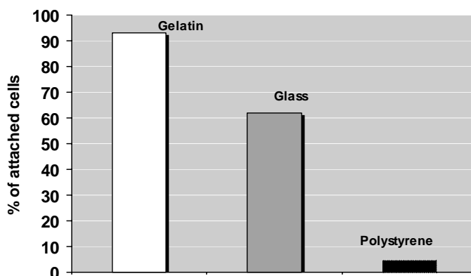
FIGURE 32.5 Attachment of fish chromatophores to gelatin, glass, and polystyrene microcarriers. Reaction conditions: L-15 media supplemented with 5% of FBS, pH = 7.4, time t = 3 h, stirring rate \nu = 40 rpm.
