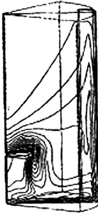
FIGURE 12.8 Typical contours of kinetic energy of turbulence using a three-dimensional model with computational fluid dynamics of an axial flow impeller (A310).
