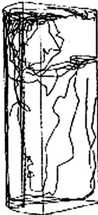
FIGURE 12.9 Typical particle trajectory using an axial flow impeller (A310) with 100 μm particles using computational fluid dynamics.
