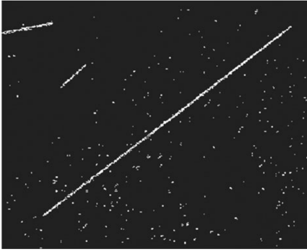
FIGURE 2.4 Optical micrograph of needle fullerene crystal structure.
