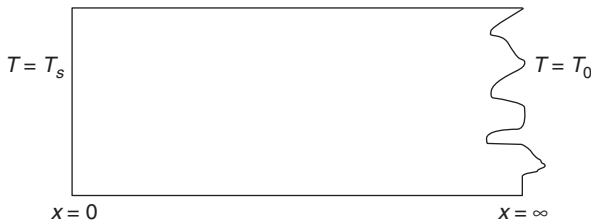
FIGURE 8.1 Semi-infinite medium with initial temperature at T_0 .
