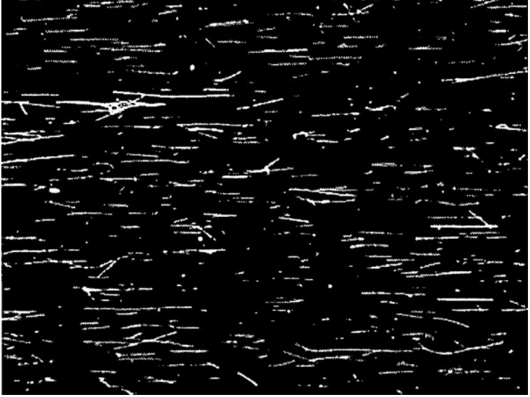
FIGURE 9.3 SEM image of nanowires (distance captured is 300 \mu\text{m} ).
