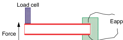
Figure 5.13 Cantilever and load-cell configuration for measuring the tip-blocking force of IPMNC samples.
