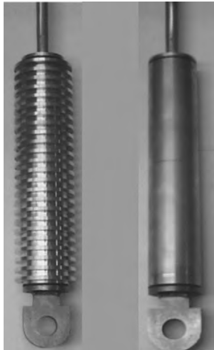
Figure 14.25 Finned (left) and unfinned (right) prototype MR-fluid dampers. 166
