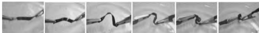
Figure 12.3 Electroinduced shape-recovery behaviour of polyurethanes–multiwall carbon nanotube composites. The sample undergoes the transition from temporary shape (linear, left) to permanent (helix, right) within 10 s when a constant voltage of 40 V is applied.
