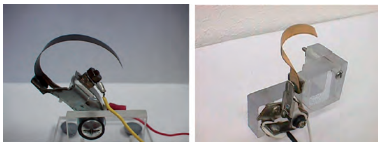
Figure 5.5 Typical deformation of strips (10 mm × 80 mm × 0.34 mm) of ionic polymers under a step voltage of 4 V.
