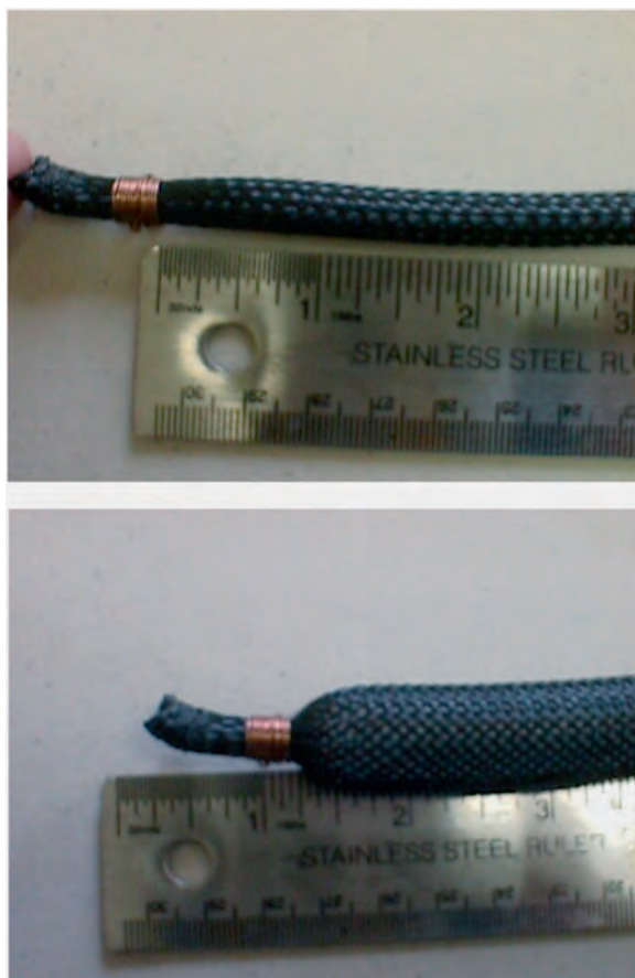
Figure 15.7 The standing position (above) and actuating (below) positions of the functioning part, respectively (this particular design gives off an approximately 20% linear strain).
