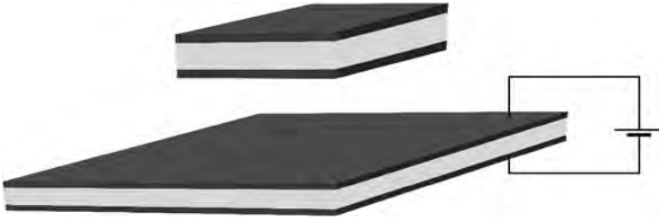
Figure 16.1 A rubbery capacitor. When a voltage potential difference is applied between the two electrodes, the pressure from the electrodes on the dielectric elastomer forces it to compress along the electric field, and expand in the perpendicular directions.
