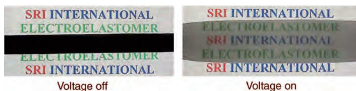
Figure 16.11 Solid-state optical aperture based on a framed actuator. The letters behind the electrode are visible only when the voltage is applied. 35
