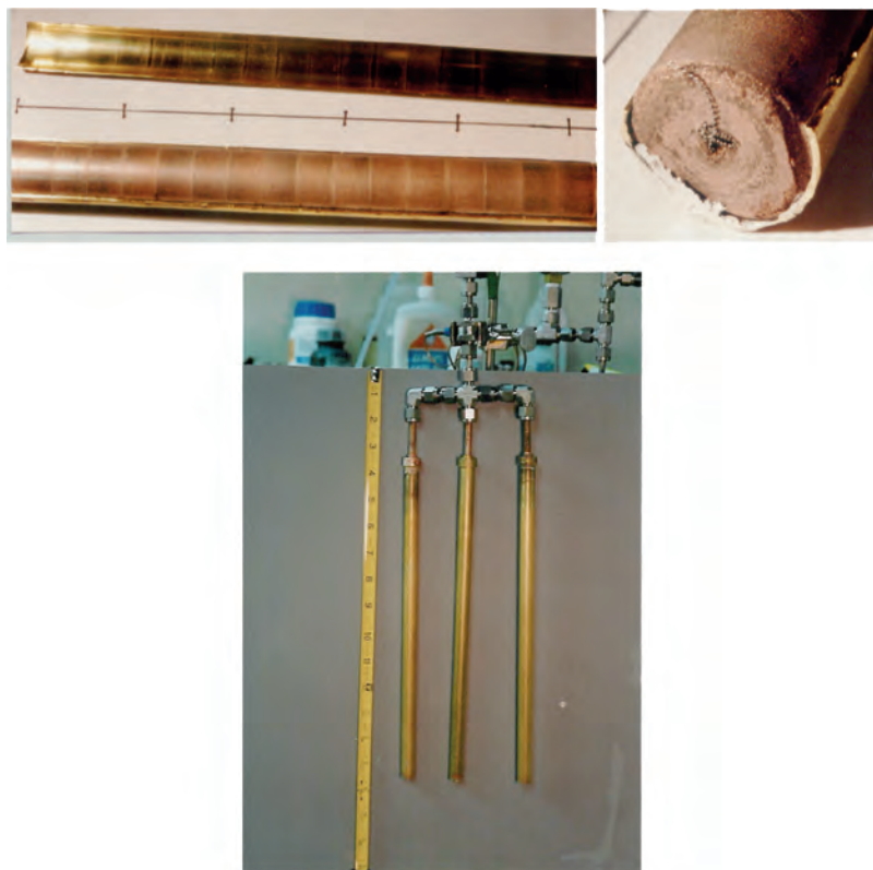
Figure 15.3 View of metal hydride, \text{LaNi}_5 , placed in a simple cylindrical container (top-left, scale is inches.) and a cross-section of the container with metal hydride (top-right). A fabricated reactor module having three reactors is shown (bottom). 2
