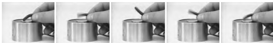
Figure 11.2 Snapshot of shape change of a magnetoelast due to modulated magnetic field. The frequency of the field is 40 Hz.
