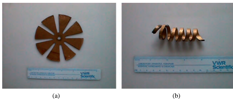
Figure 5.1 (a) An eight-finger synthetic muscle. It has a thickness of approximately 2 mm; (b) A coil-type synthetic muscle. This coil type muscle creates a linear actuation motion.
