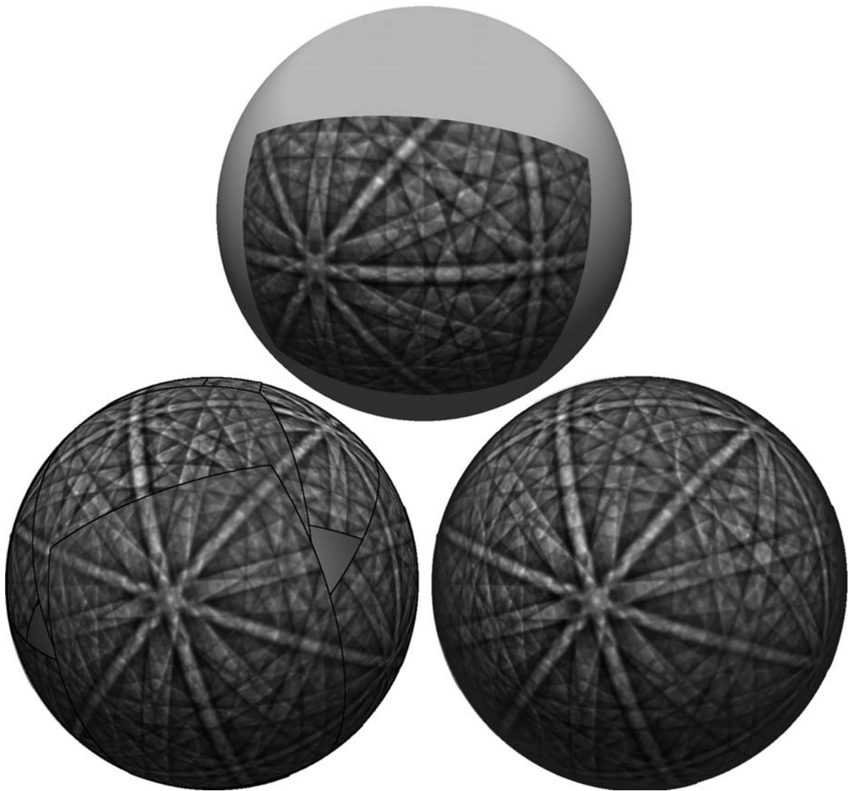
Fig. 5.7 Example showing the creation of a spherical Kikuchi map; starting with a single fcc EBSP ( top ); repeating it using symmetry ( left ); and adding in other EBSPs at different orientations with averaging ( right )
