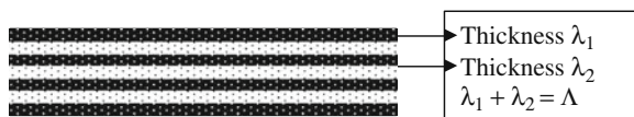
Fig. 1 A Schematic of a compositionally modulated material consisting of two different components. The individual thickness of each layer is \lambda_1 and \lambda_2 . The overall modulation thickness is the sum of the individual thicknesses, \Lambda
