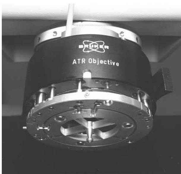
Figure 1.10 Photograph of the Bruker Optics ATR objective. Illustration courtesy of Bruker Optics.
