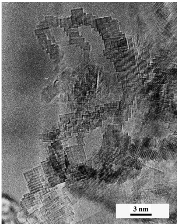
Figure 14.3. HRTEM image of nanoscale MgO (AP-MgO). Reprinted from Ref. 20 with permission.
