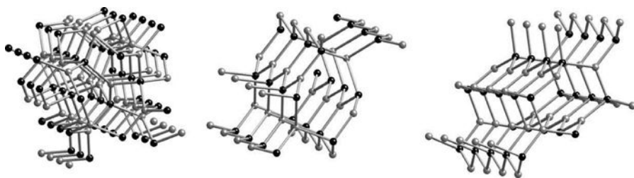
Figure 22.14. Idealized structures of three \text{Si}_3\text{N}_4 polymorphs (4): (left) cubic, (center) tetragonal, and (right) hexagonal. The black spheres correspond to Si atoms and the gray ones to N atoms.
