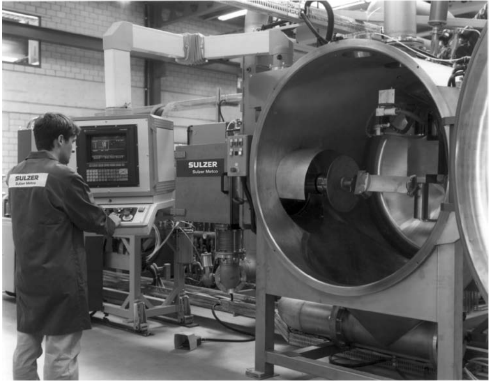
Fig. 5.9. Commercial vacuum plasma spraying (VPS) equipment for the production of thermally sprayed coatings. (Courtesy of Sulzer Metco.)
