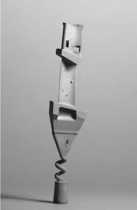
Fig. 3.5. Rolls-Royce Trent 800 high-pressure turbine blade casting, after removal of the investment shell.
