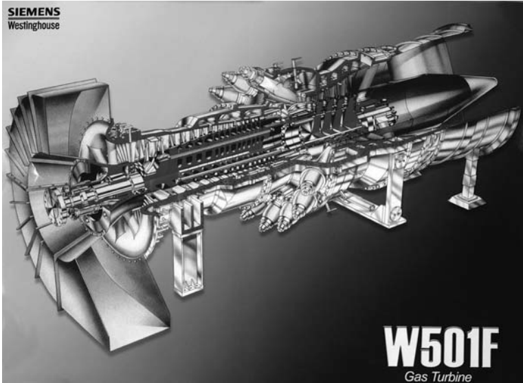
Fig. 1.2. Artist's impression of the turbomachinery in Siemens Westinghouse's W501F gas turbine engine, used for electricity generation. (Courtesy of Siemens Westinghouse.)
