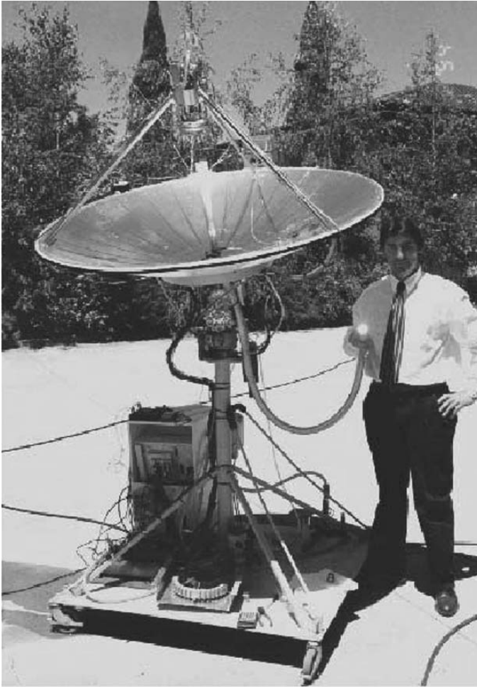
Fig. 8. This photo, taken in the 1990s, shows John Lasich demonstrating how cool his concept is for conducting infrared energy through a fiber-optics light pipe. The dish reflects sunlight to a “heat mirror” that reflects long-wavelength solar radiation to the fiber-optic bundle along the axis of the parabolic dish. The visible light seen at the end of the light pipe in Lasich’s hand is a result of partial reflection of visible light by the heat mirror.
