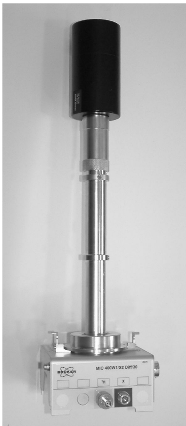
Figure 5.1 A specialised high z -gradient diffusion 400 MHz heteronuclear probe capable of generating gradients up to 30 \text{ T m}^{-1} when coupled to a suitable gradient amplifier (i.e., providing a current of 60 A). The entire gradient coil consists of various individual cylindrical coils in a multilayer design with channels for water cooling. The inner diameter of the gradient system (black cylinder at the top of the probe) is 19 mm. The probe can be configured with fixed or with exchangeable rf-coils up to 10 mm inner diameter. By changing the gradient set to one containing three orthogonal x - y - z -gradient coils, the same probe can be used for investigating anisotropic diffusion and for imaging studies. In this case the maximum gradient strength gets reduced to 3 \text{ T m}^{-1} at currents of 60 A. Photo courtesy of Bruker Biospin.
