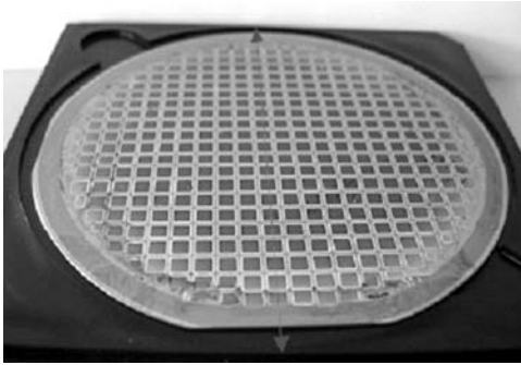
Figure 19.1 Fully etched 4-inch Si wafer with PSi areas (darker gray) and bulk Si bridges in between (light gray). The partial etching is realized by masking the wafer with silicon nitride (this image was taken by CiS Institute for Microsensorics, from the “SilAnz” report [14]).
