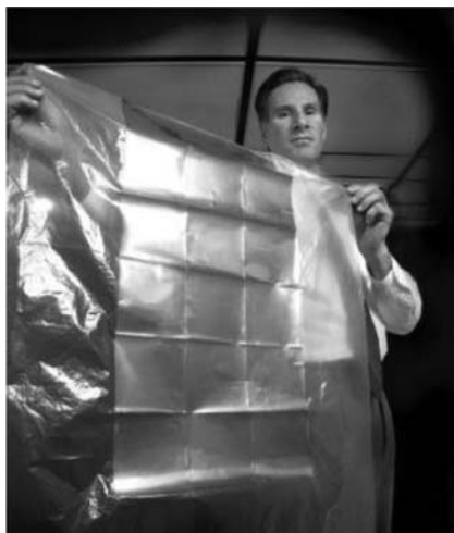
Figure 6.20 INL researcher Steven Novack holds a plastic sheet of nanoantenna arrays, created by embossing the antenna structure and depositing a conductive metal in the pattern. (Photo courtesy: Idaho National Laboratory).
