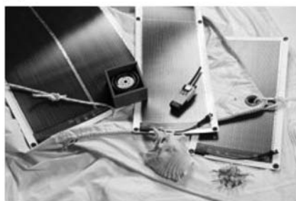
Figure 1.2 Plastic solar cells such as (a) that entirely organic (Photo courtesy: Konarka) or (b) that using amorphous Si (Photo courtesy: Flexcell) are lightweight ( 25\text{--}50\text{ g m}^{-2} ), and ideally suited for customized integrated solutions.
