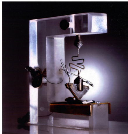
Figure 1.8 A photograph of the first transistor (Courtesy of The Porticus Centre).
