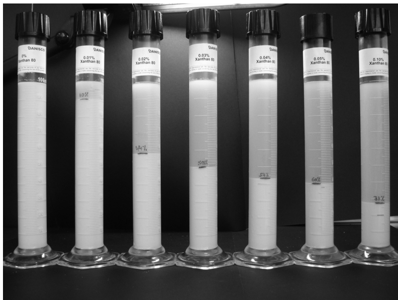
Fig. 5.14 Phase separation after addition of xanthan gum to semi-skimmed milk. For a colour version of this figure, please see the colour plate section.
