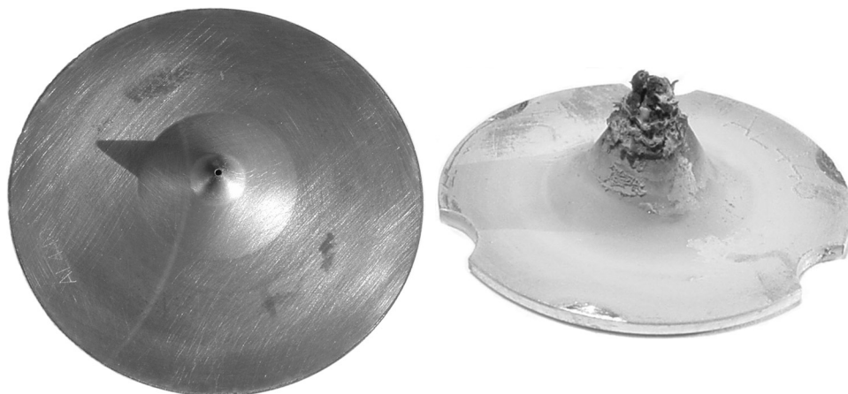
Figure 4.1 Concentrated solution of digested, freeze-dried plant material (~120 mg in ~23 mL of 2% nitric acid) leads to blockage of the cooler skimmer cone (right) while the hotter sample cone shows no deposits (left).
