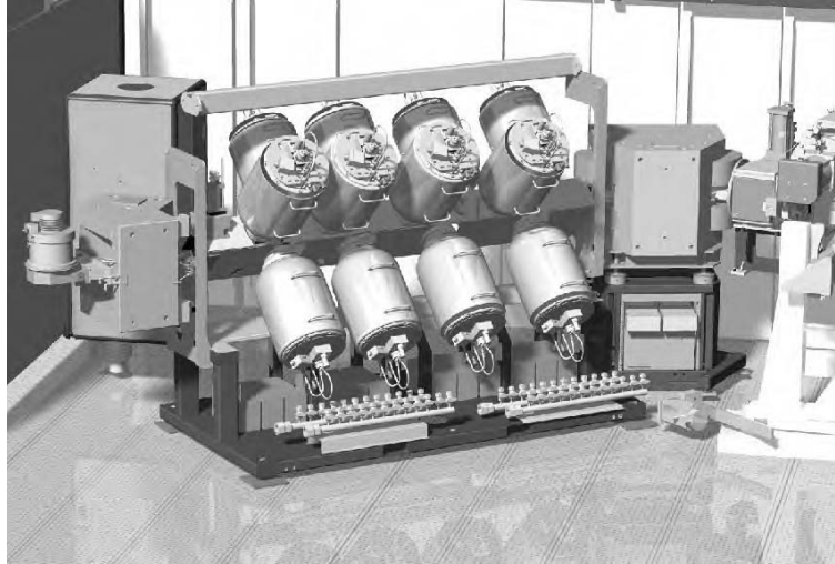
Fig. 15.4. High energy beamline featuring an RF linac with 12 resonators. The ion source and analyzer magnets are on the left. The final energy magnet is on the right
