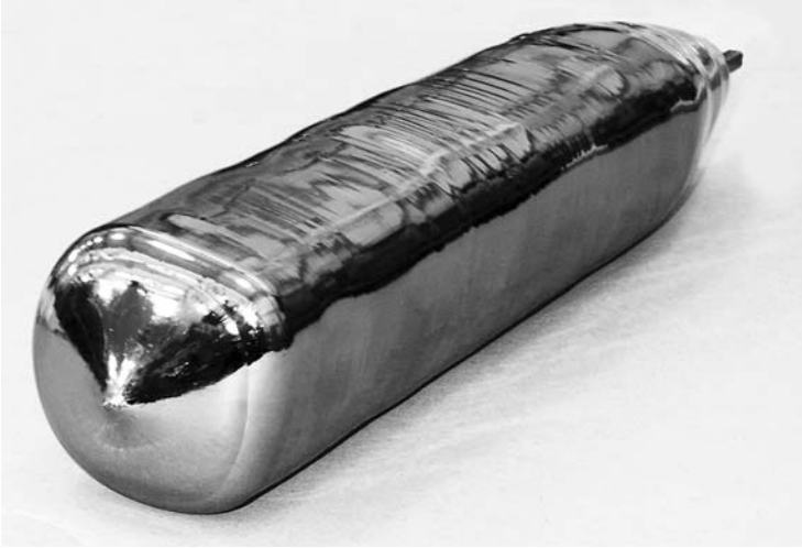
Fig. 3.8. qFZ crystal with almost quadratic cross section ( 100 \times 100 \text{ mm}^2 , rounded). The instabilities at the sides and the deviation from the square shape can be seen
