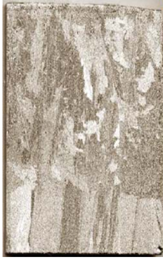
Fig. 1.15. Picture that shows breakdown of the solidification front in MC Si
