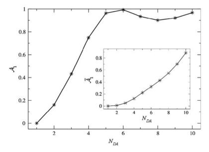
Fig. 6 The current asymmetry factor  $A_1$  as a function of the number of links,  $N_{DA}$  connecting the D and A wires in the DA system displayed in Fig. 4a. The *inset* shows the same data, presented in terms of  $\overline{A_1}$  plotted as a function of  $N_{DA}$ . Parameters are similar to those in Fig. 5
