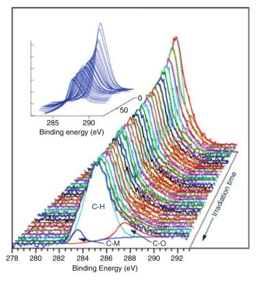
**Fig. 8** Series of C 1s XPS spectra of (*R*)-2-butanol adsorbed on permalloy obtained sequentially while irradiating with 1,190-eV X-rays. The *inset* shows the area of the C–O peak component as a function of irradiation time
