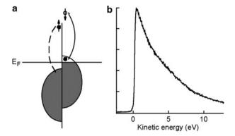
**Fig. 2** (a) Schematic illustration of the way preferential scattering of minority electrons leads to a net spin polarization of the majority electrons in the production of secondary electrons in a ferromagnet. (b) Representative secondary electron yield curve from permalloy excited with 1,190 eV X-rays
