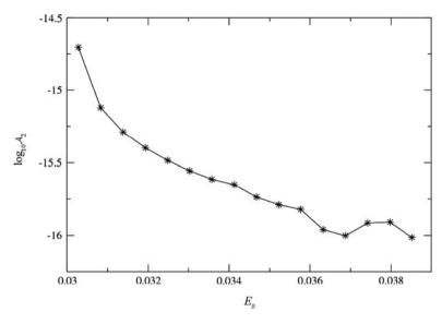
**Fig. 8** The current asymmetry factor  $\mathcal{A}_2$  as a function of the bridge site energy  $E_B$  for the DBA system in the off-resonance regime,  $E_B > 0.03$ . The parameters used in this calculation are  $E_D = E_A = 0$ ,  $\beta_D = \beta_B = \beta_A = 0.1$ ,  $V_{DB} = V_{BA} = 0.01$ , E = -0.17,  $N_{DB} = 3$ ,  $N_B = 2$ ,  $N_{BA} = 2$ . Coarse grained averaging was used to reduce numerical errors that results from computing small differences between relatively large numbers
