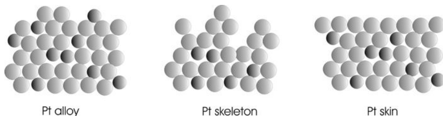
FIGURE 4 Three different nanostructures of \text{Pt}_3\text{M} alloys.
