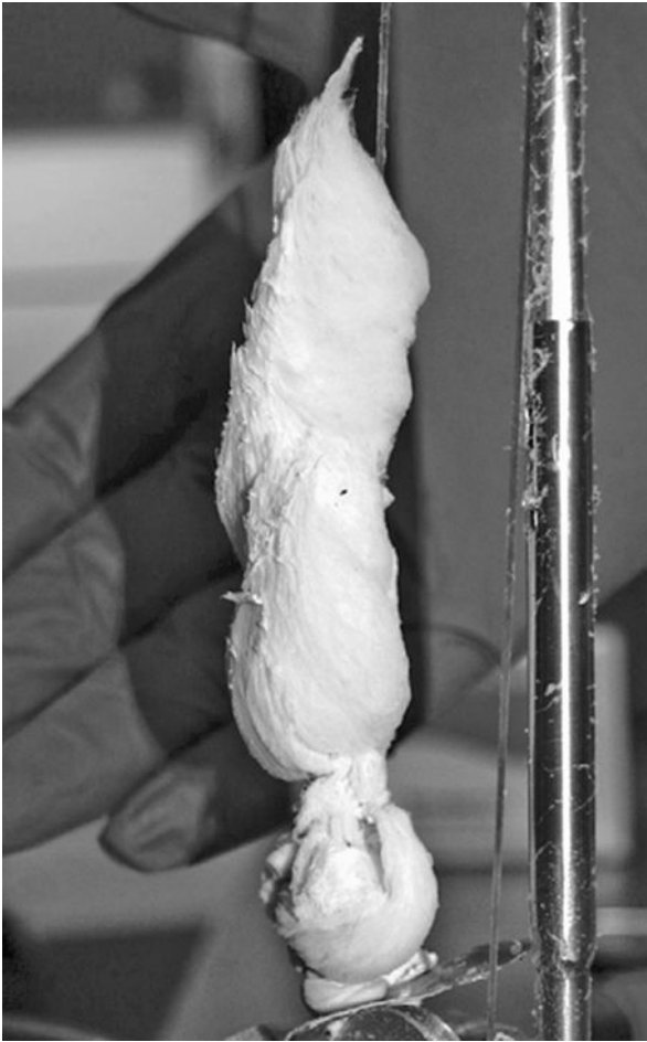
FIGURE 26 BN nanotube product formed by continuous laser ablation. (Reprinted from [42] with permission of IOP © 2009.)
