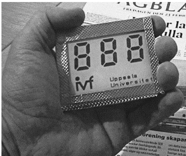
Figure 11.5 Prototype electrochromic display showing an ‘electric paint’ display: the primary electrochrome was viologen ( IV ) adsorbed on nanocrystalline \text{TiO}_2 . (Figure reproduced from Pettersson, H., Gruszecki, T., Johansson, L.-H., Edwards, M.O.M., Hagfeldt, A. and Matuszczyk, T. ‘Direct-driven electrochromic displays based on nanocrystalline electrodes’. Displays , 25 2004, 223–30, with permission of Elsevier Science Ltd.)
