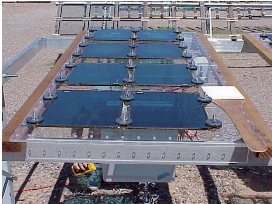
Plate 7 Gentex windows being tested in Florida. A man is just visible beneath the nearest. (Reproduced with permission from Rosseinsky, D.R. and Mortimer, R.J. 'Electrochromic systems and the prospects for devices'. Adv. Mater. , 13 , 2001, 783-93, with permission of VCH-Wiley.)
