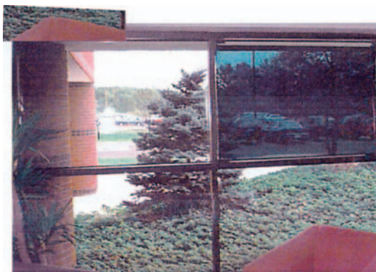
Plate 4 Gentex window of area 1 \times 2 \text{ m}^2 . The top right pane has been electrocoloured. The other three panes are bleached. (Reproduced with permission from Rosseinsky, D. R. and Mortimer, R. J. 'Electrochromic systems and the prospects for devices'. Adv. Mater. , 13 , 2001, 783–93, with permission of VCH–Wiley.)
